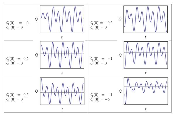
The fact that all these solutions begin differently but settle down to the same long-term behavior suggest the following terminology: the behavior of Q(t) near t = 0 is called the *transient behavior*, while the wave form that it settled down to after some time is the *steady state*. The steady state does not depend on the initial conditions; it only depends on the wave V(t) being fed into the circuit.
