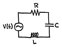
The picture below shows the three components mentioned arranged in sequence (before they are connected to a power source). In this picture, the order is resistor, inductor, capacitor, although as I mentioned the order of the components does not affect the behavior of the circuit.
